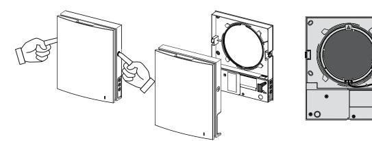
5 - Mount the Electronic Component Secure the electronic unit using the provided screws.
