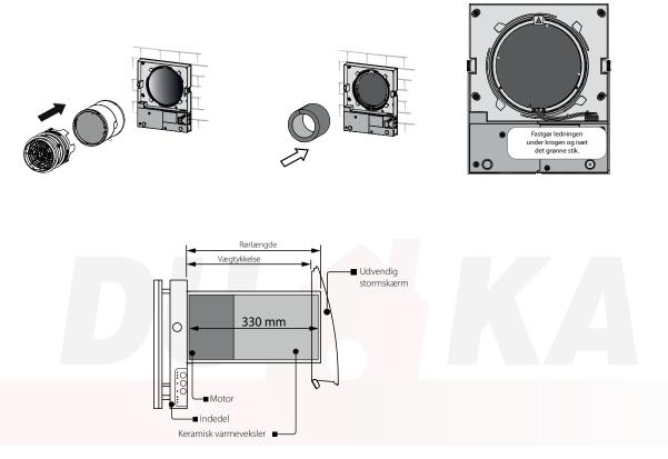
Note: Reducing the distance between the motor and exchanger may affect performance and noise levels.
