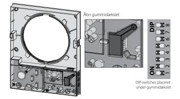
Before starting the DUKA One unit, the operating settings must be adjusted to fit your needs. This is done using the DIP switches, located under the DIP switch cover.
